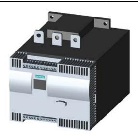
SIRIUS SOFT STARTER, VALUES WITH 460 V, 50 DEG., STANDARD: 215A, 150HP, INSIDE-DELTA CIRCUIT 3: 372A, 300HP, 200-460 V AC, 115 V AC, SCREW TERMINALS
